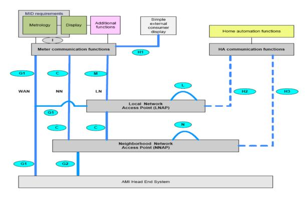
The diagram above is taken from TR 50572 and gives a simplified overview of functional entities and interfaces in a smart metering communications network; the boxes correspond to functions that in physical terms can be implemented in a number of different ways. TR 50572 is concerned solely with the communications interfaces depicted in blue.
